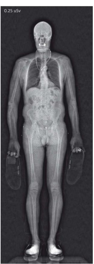
A typical image from Intercept on the lowest setting, 0.25 uSv. Items: teeth fillings, neck chain, object in shoe heal, ring and zipper. Intercept can operate at up to 200 uRem for even better image quality.
